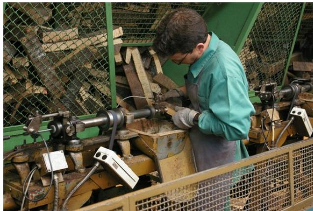
*Figure 4: Hand-punching bottle stoppers [3]*
